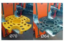
The forks pick up trolleys of different sizes
