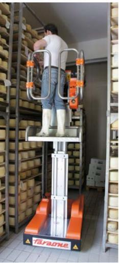
QUICK AND EASY TO USE It is extremely easy to handle with quick selfpropulsion: 5 km/h at top speed. It has a zero turning circle.
